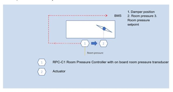
◆ For room pressure control and air flow measurement
